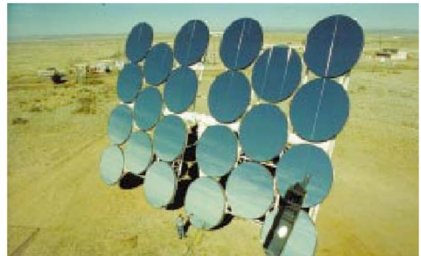
A new SAIC faceted membrane heliostat is on test at the National Solar Thermal Test Facility.
