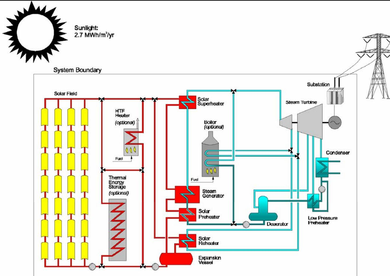
Figure 1. Solar/Rankine parabolic trough system schematic [1].
