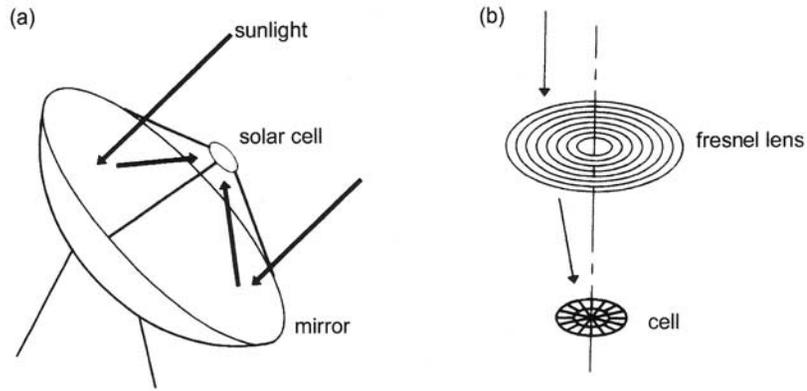
Fig. 7.5 Point-focus systems with rotational symmetry, (a) Dished parabolic mirror; (b) Fresnel lens
