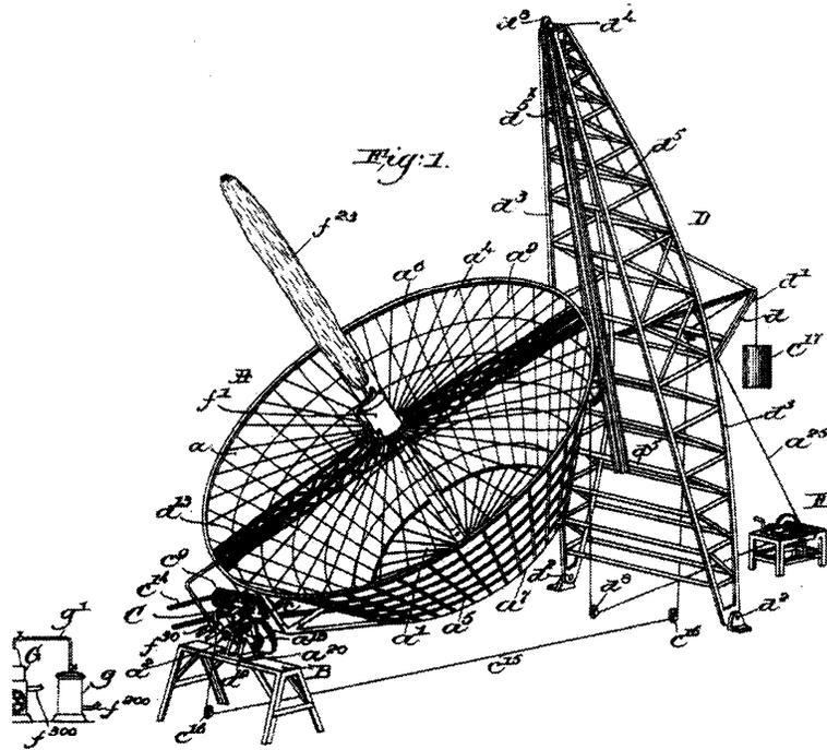
Patent drawing for Aubrey Eneas's second solar motor, 1899. To follow the sun's motion, the truncated cone mirror was moved along a track in tower scaffolding at right.
