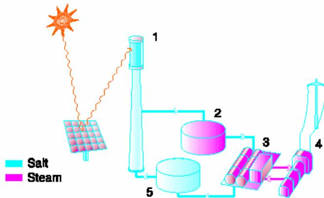
Schematic of electricity generation using molten-salt storage:
