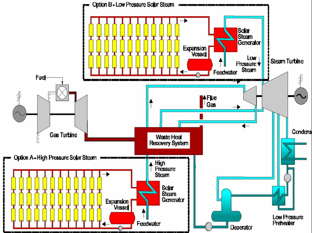
Figure 2. Integrated Solar Combined Cycle System [1].
