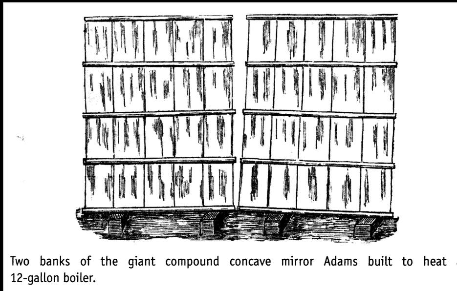
Two banks of the giant compound concave mirror Adams built to heat a 12-gallon boiler.
